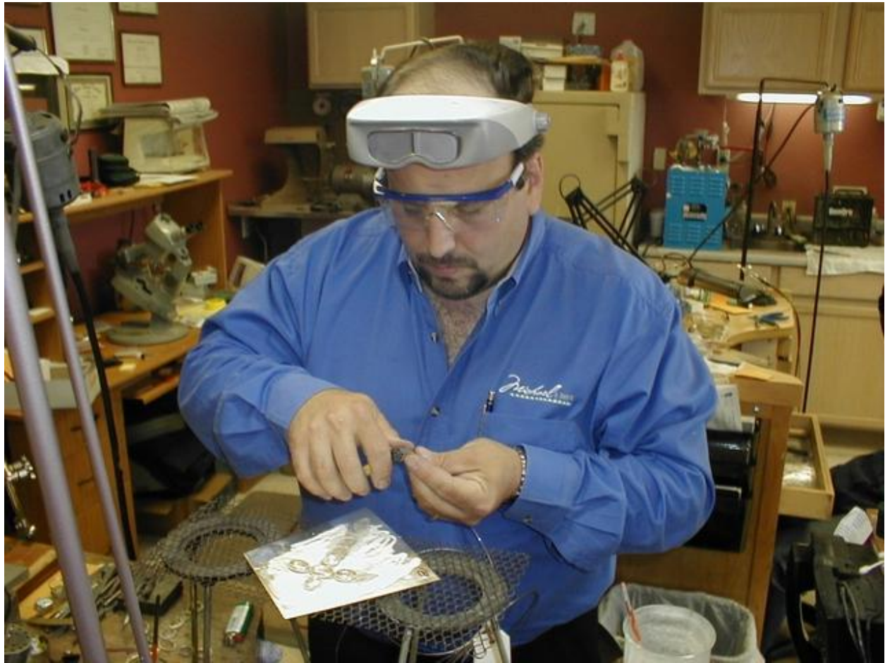
Snipping solder as David solders the bezels and twisted bezel wire rings to the 18 gauge plate that will serve as the backbone of the cross
