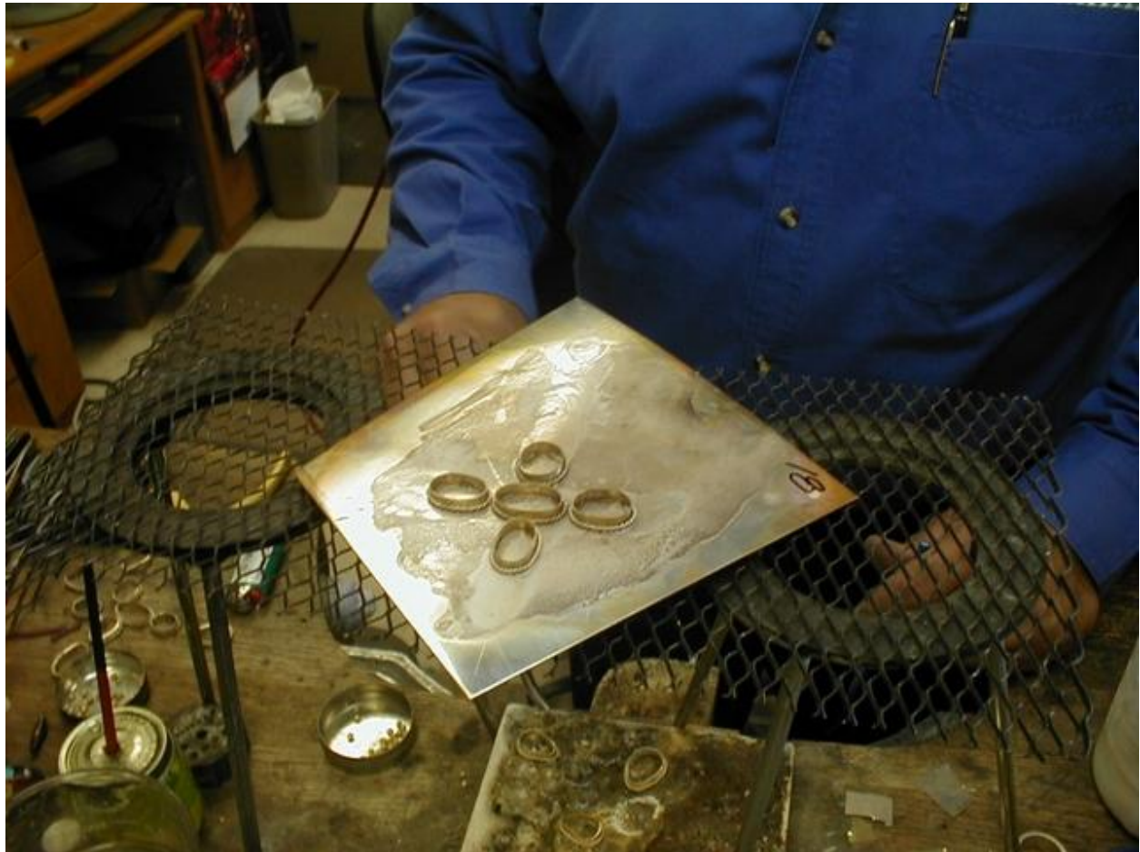
A closer look at the work being done as David solders more bezels in place.
